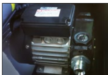
Automatic-manual fuel transfer pump
