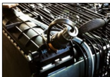
Coolant level sensor in radiator
