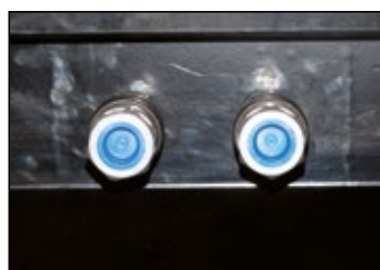
Fast fuel plug connection between external and internal fuel tank.
